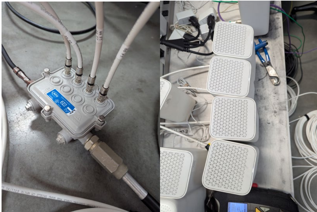
Figure 8 – 4 Test Modems and Their High-Value Tap Connections
