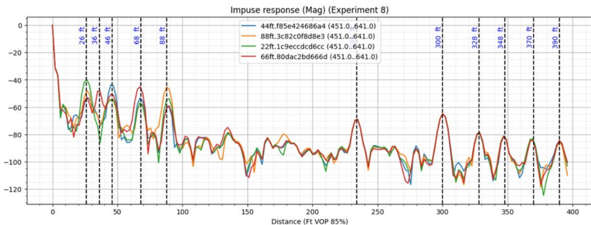
Figure 45 – Experiment 8, Time-Domain Impulse Response, 400 Feet
